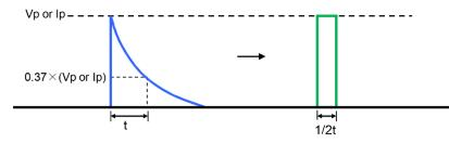
2. Damping oscillation wave with time constant of envelope "t"  $\rightarrow$  Square wave
